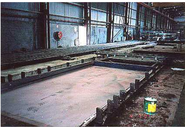
Figure 9. Adjustable Steel Mould
