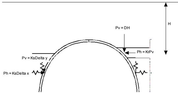
**Figure 4: Beam and Spring Analysis**
