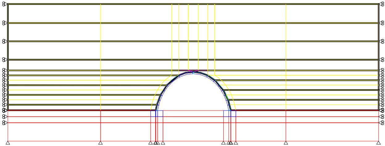
Figure 2: Finite Element Mesh
