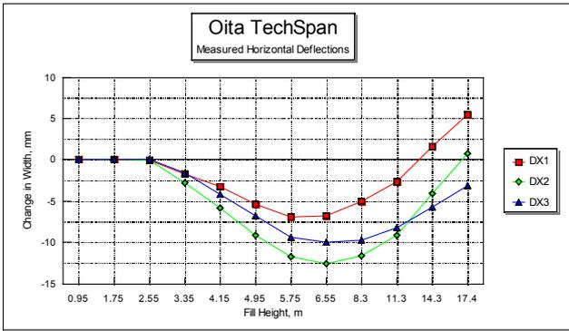
Figure 6: Measured Horizontal Deflections
