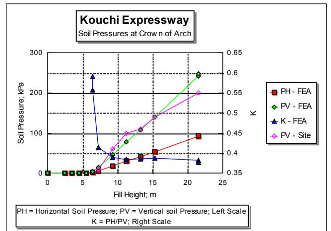
Figure 17; Soil pressures at crown
