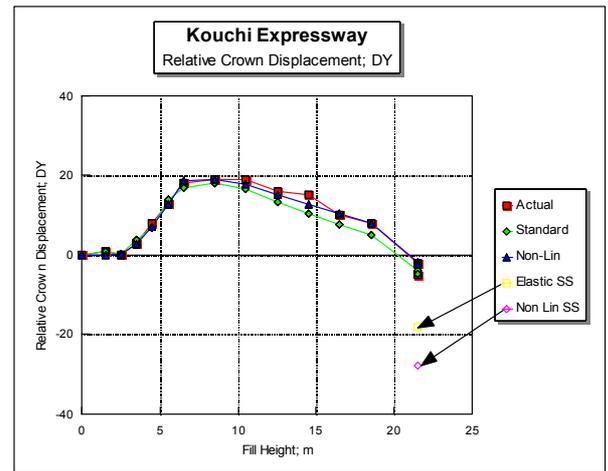
Figure 9; Vertical deflection at crown
