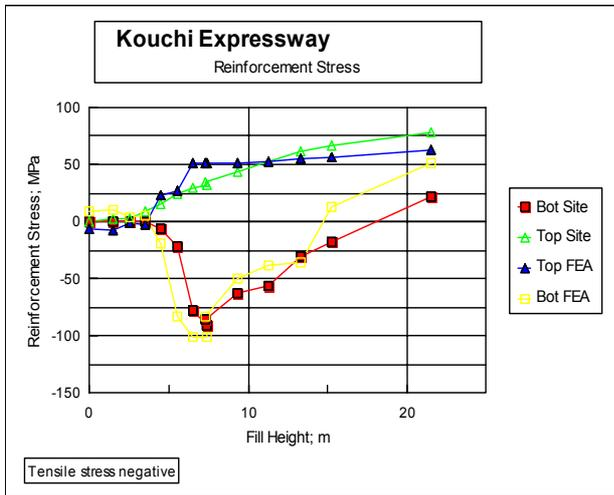
Figure 13; Reinforcement stress
