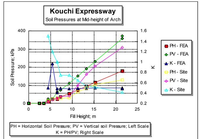
Figure 16; Soil Pressures at mid-height
