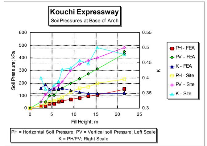
Figure 15; Soil pressure at base
