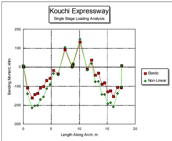
Figure 12; Bending Moment, single stage loading
