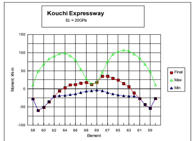
Figure 10; Bending Moment Envelope,  $E_c=20GPa$
