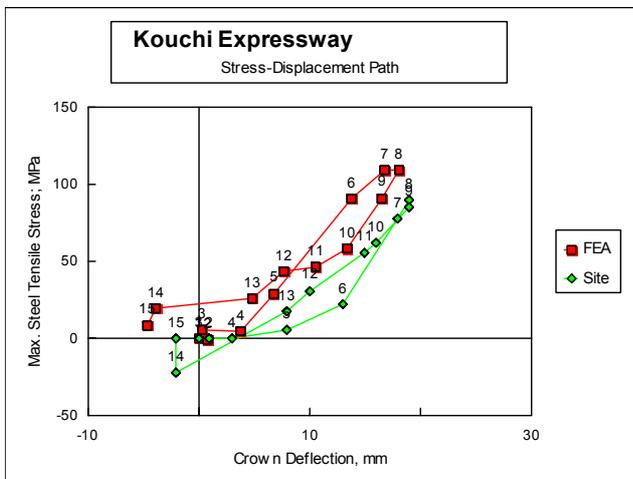
Figure 14; Stress-displacement path
