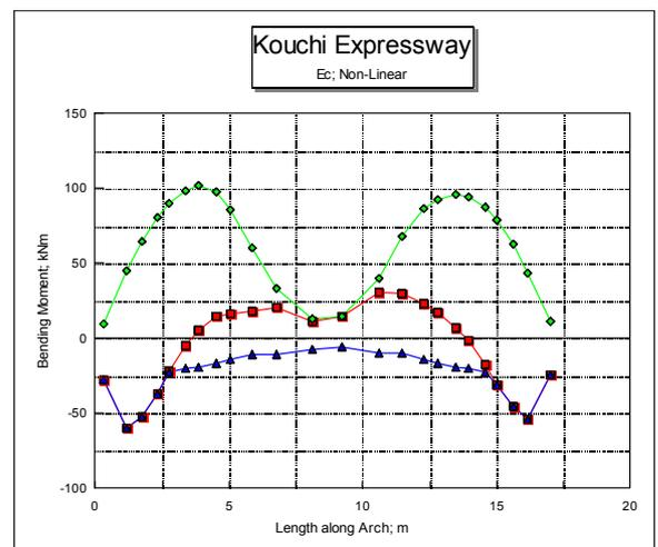
Figure 11; Bending Moment Envelope, Non-linear  $E_c$
