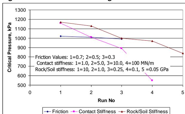
Figure 5: Effect of contact friction and stiffness and Rock/Soil stiffness
