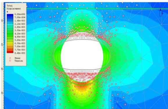
Figure 7: Stage 4 - Current State of Stress
