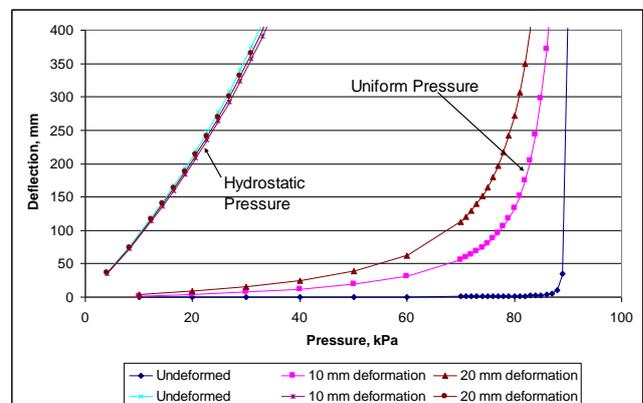
**Figure 2: Unrestrained Buckling - deflection**
