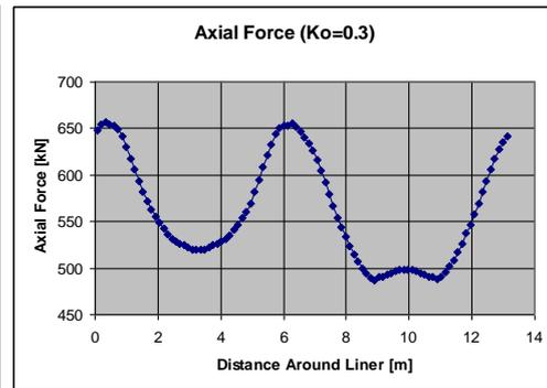
Figure 9: Bending Moment transfer to Steel liner Figure 10: Axial Load Distribution in steel liner
