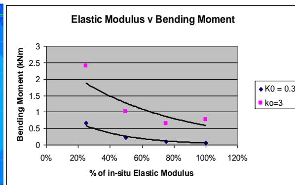
Figure 8: Effect of Elastic Modulus on Load Shed
